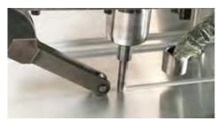
Joining the metal using the FSW technology
